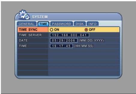
If the DVR is connected to the network, and if there are more than one DVR connected, then a DVR can be configured as the master DVR from which all other DVRs synchronize their time and date. The default is OFF.
