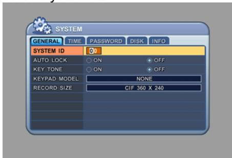
Select the DVR's SYSTEM ID. Up to 99 DVRs can be controlled using one remote controller. To select the DVR to be controlled with the remote controller, press and hold the DVR ID button. While holding the DVR ID button, press the appropriate DVR ID number. For example, enter 05 for DVR ID 05, enter 43 for DVR ID 43, and such. The default value is 0.
