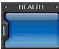
The color remains blue as long as the DVRs are functioning within the normal parameters. It will display the DVR's set name only with the following functions: recording started, backup started and schedule on.
