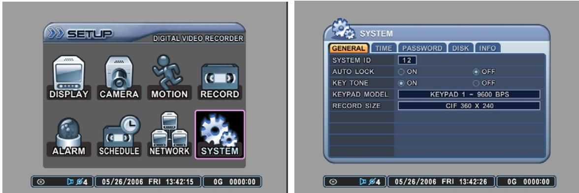
System Setup allows modification of various system features such as System ID, Automatic Key Lock, Key Tone, HDD rewrite policy, overall system record resolution, Time and date related settings, Password for different levels of users, formatting various hard disk drives and the system information.
