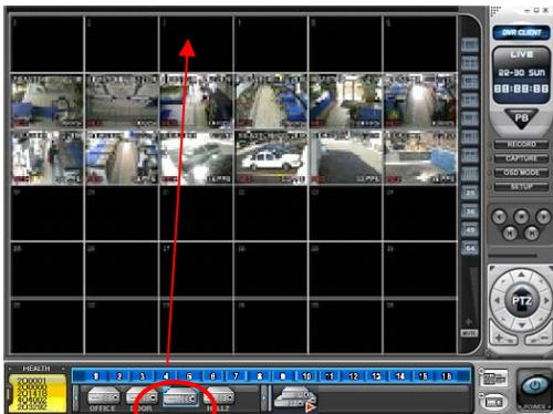
Individual cameras can be added onto the Virtual DVR by click-and-dragging individual cameras.
