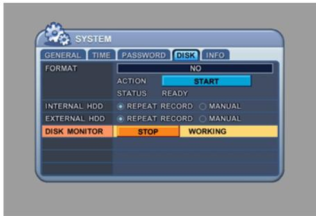
By factory default, the DVR is consistently monitoring the HDD for any malfunction and failures. You can manually turn this function off. **This feature is not supported.**
