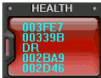
The color changes to red when critical functions of the DVR is interrupted or has failed: connection failure, connection timed out, disconnection, power failure, fan lock/recovery, system failure/recovery and HDD failure/recovery.
