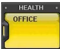
The color changes to yellow when recording and alarm related events occur: video loss, video loss recovery, alarm trigger, motion detection, recording stopped, schedule off and backup stopped.
