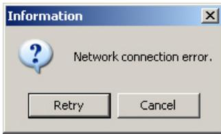
If the icon is double-clicked while the DVR is disconnected or if the password has been changed on the DVR, “Network connection error.” pop-up window will appear. Click on **Retry** to reinitialize the connection process or **Cancel** to return to the main window.
