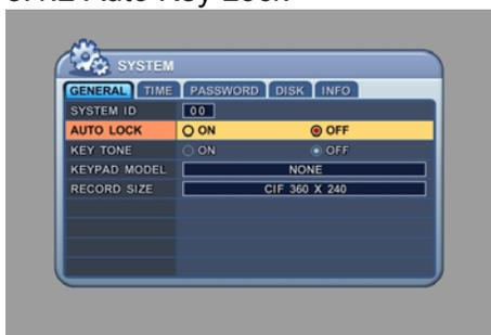
The DVR locks all the buttons after three minutes of inactivity. The buttons can be unlocked with the user password. The default is OFF.
