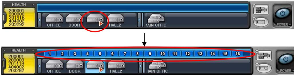
Once the cameras are displayed on the bar, any of the cameras may be double-clicked to display the selected camera in single channel mode.
