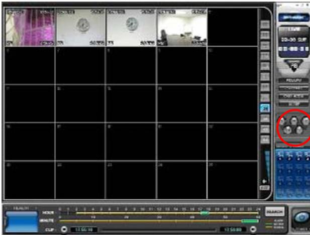
Once the playback begins, the video can be manipulated using the playback controls. The video can be fast forwarded, fast rewind, paused, move field by field in either direction.
